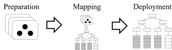
Fig. 4: Workflow for embedding of VN request.
